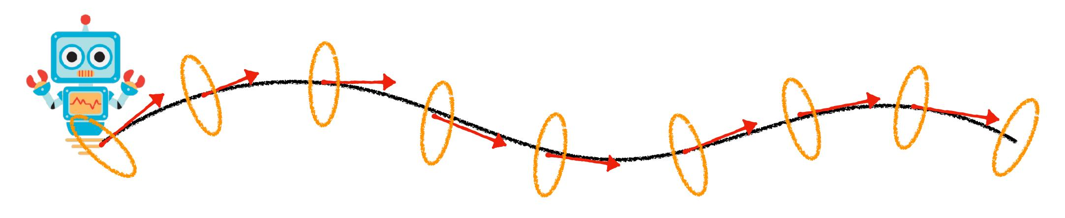
Step 1: Forward pass - roll out current guess u(t)Step 2: Linearize dynamics, quadricize cost around roll out Step 3: Backwards pass - compute LQR gains  $K_t$  at each time
