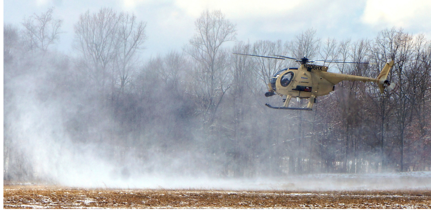
Figure 1: Boeing Unmanned Little Bird (equipped with TALOS system) executes an autonomous landing on snow.
