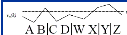
Figure 3: Determining word boundaries. The X-Y boundary is created by the threshold criterion, the other three by the local maximum condition.
