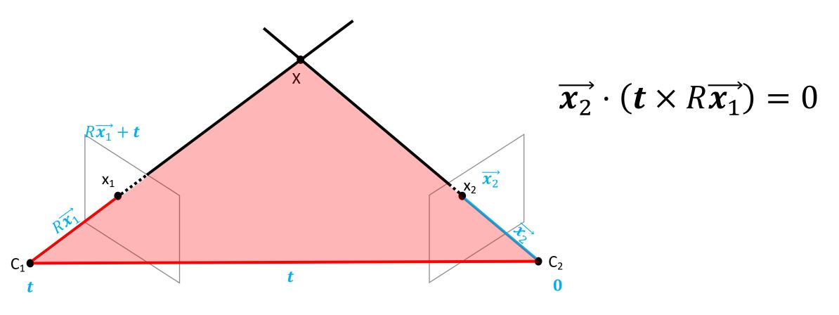
$$\vec{\mathbf{x}}_{img}^{(2)} \cdot \mathbf{t} \times R \vec{\mathbf{x}}_{img}^{(1)} = 0$$
