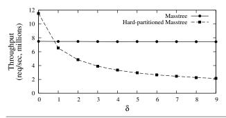
**Figure 11.** Throughput of Masstree and hard-partitioned Masstree with various skewness (16-core get workload).
