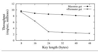
**Figure 9.** Performance effect of varying key length on Masstree and "+Permuter." For each key length, keys differ only in the last 8 bytes. 16-core get workload.
