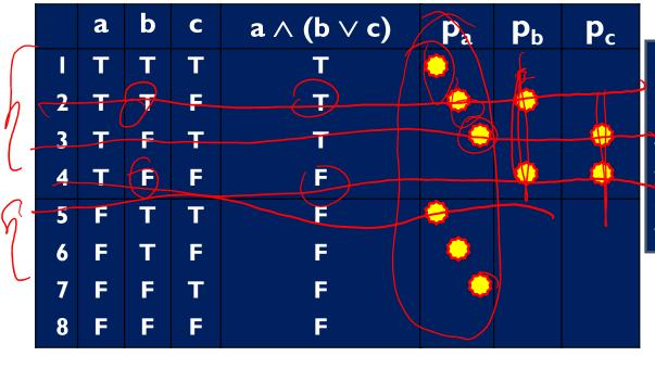
In sum, three separate pairs of rows can cause a to determine the value of p, and only one pair each for b and c
