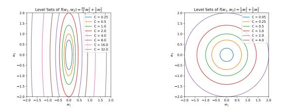
Main idea of preconditioning: rescale the underlying space we're optimizing over to make the level sets more like circles. To do this for an objective function f, let's imagine solving the modified optimization problem where we minimize g(u) = f(Ru) for some fixed matrix R. Gradient descent for this task looks like
