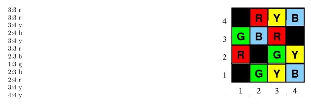
Here, the robot begins in square 3:3 perceiving red, attempts to make an illegal move (to the right), so stays in 3:3, still perceiving red. On the next step, the robot moves up to 3:4 perceiving yellow, then left to 2:4 perceiving blue (erroneously), and so on.
