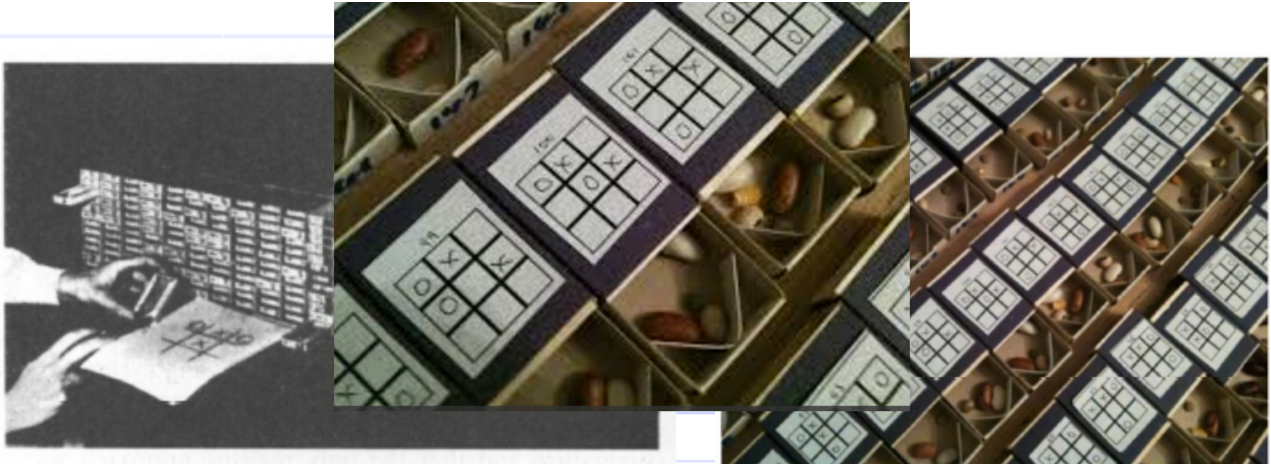
Fig. 2.—The matchbox machine—MENACE
