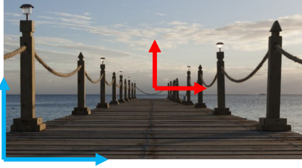
Figure 3: The image coordinate system must be changed from the one shown in red, to the one shown in cyan.
