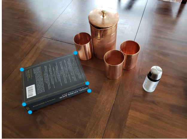
Figure 1: Input for camera calibration. For the cyan points, we also know corresponding world coordinate locations.
