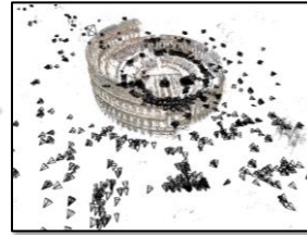
Reconstructed 3D cameras and points
