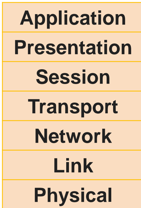
Proposed 7-Layer ISO/OSI reference model (1970's)
