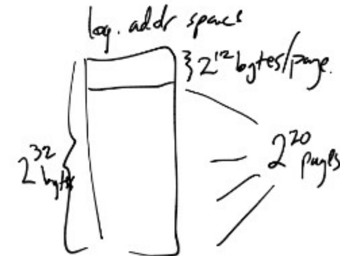
$$\begin{aligned} & 2^{20} \text{ entries} \cdot \frac{4 \text{ bytes}}{\text{entry}} : 2^{22} \text{ bytes in PT.} \\ & = 4 \text{ MB / PT} \end{aligned}$$
