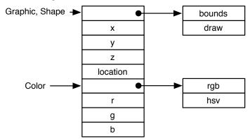
There are two distinct "views" of the object, one as either a Graphic or a Shape, and one as a Color. To switch between these views, some computation is required. For example, we might subsumption to view a Graphic as a Color:
