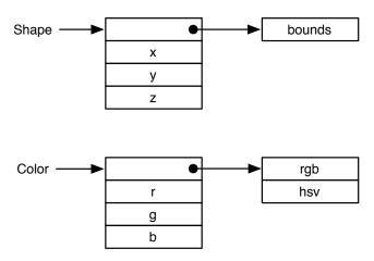
We can merge both these layouts into a single object, but we need separate dispatch tables because bounds() and rgb() use the same method index:
