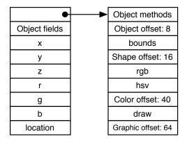
The sequence to access a field is more expensive than the usual indexed load. Before multiple inheritance, an access like of could be implemented as  $movk_f(o)$ , t, where  $k_f$  is a known constant offset. With this object layout, accesses are more complex:
