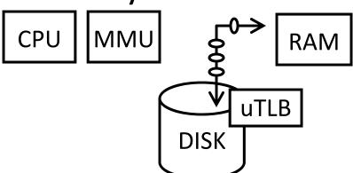
Solution 2: DMA uses virtual addresses
