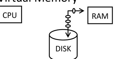
Solution: Pin the page before initiating DMA Alternate solution: Bounce Buffer
