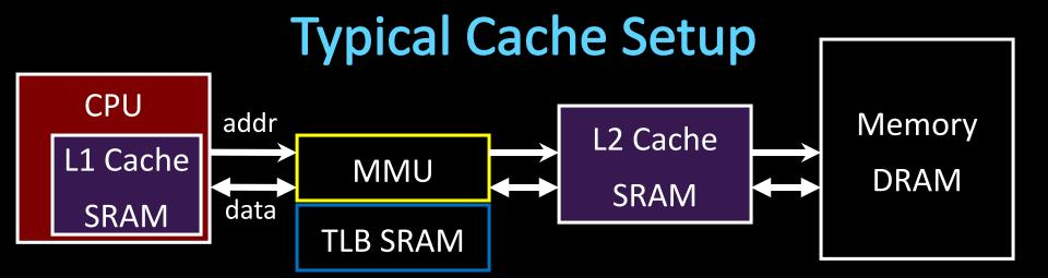
Typical L1: On-chip virtually addressed, physically tagged
