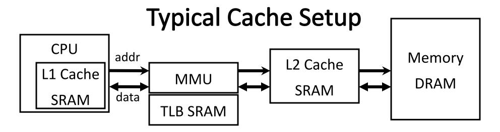
Typical L1: On-chip virtually addressed, physically tagged
