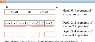
Max depth: about log n. Time to partition on each level:  $\sim n$  Total time: O(n log n).
