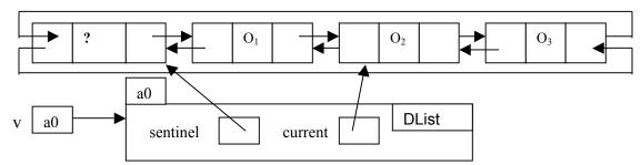
A variable v that represents a list is of class DList. An instance of DList has a field sentinel that is the name of (or a pointer to) the header node, which is an instance of DNode. The header always exists. *The value of the header node is irrelevant to this question and should not be tested.* If the list of items is not empty, field current contains the name of a node for some item.
