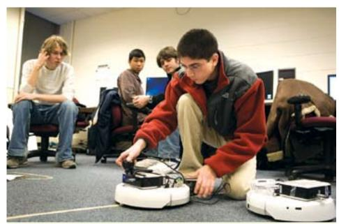
Kamran Munshi fine-tunes his team's robot before a demonstration of its programming to follow a pattern on the floor. The addition of a compact computer and a video camera gives the basic iRobot more sophisticated capabilities.
