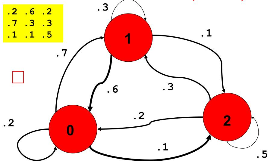
Computing the Stationary Array Involves a Probability Array
