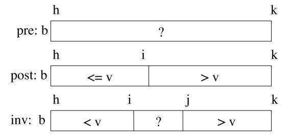
Called binary search because each iteration of the loop cuts the array segment still to be processed in half
