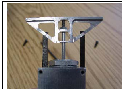
Figure 6-11 The plastic guide would restrict kicker rotation effectively
