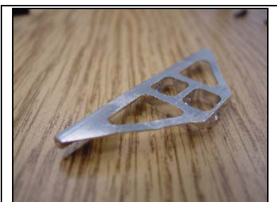
Figure 6-6 Bottom view of finished kicker
