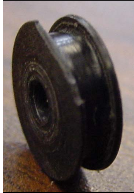
Figure 2-28 Fractured Delrin Roller
