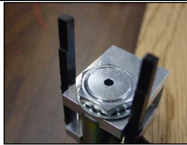
Figure 6-9 Top view of solenoid mount, with locking hex nut
