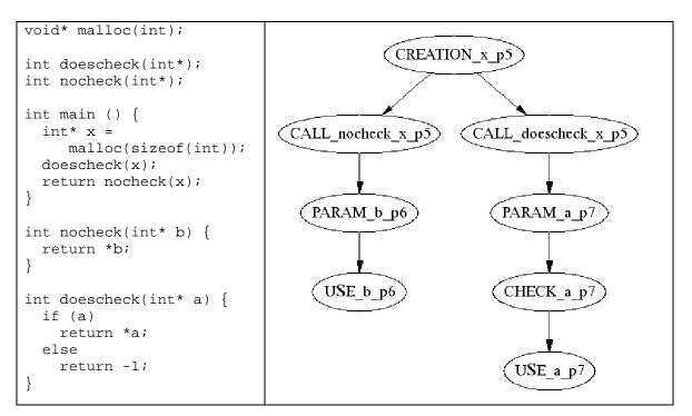
As an example, the null-paths prototype was run on the C code below on the left to generate the graph on the right.
