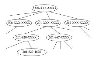
Figure 1 Fixed-position address hierarchy (with decimal addresses)
