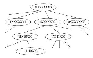
Figure 2 Variable-position address hierarchy (with binary addresses)
