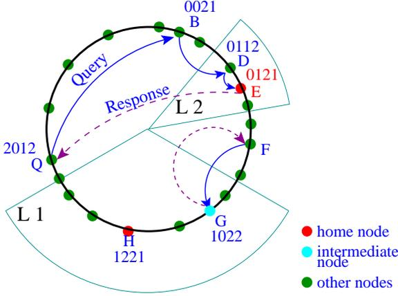
Figure 1: CobWeb Replication on top of Pastry.
