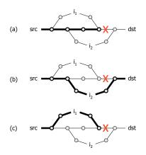
Figure 6: **Disjoint paths.** (a) The default path to the destination fails due to a faulty link. (b) Routing through intermediary  $i_2$  would succeed, since the diverted path is disjoint from the faulty link. (c) Routing through intermediary  $i_1$  would fail, since the diverted path rejoins the default path before the faulty link.
