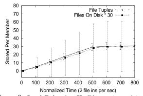
Figure 3: Load Balancing II: Files are inserted into a 1000 node system (30 affinity groups), 2 insertions per sec between t=0 and t=500. Plot shows variation, over time, of number of files and filetuples at a node (average and one standard deviation).
