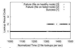
Figure 5: Fault-tolerance of Lookups I: In a 1000 node (30 affinity groups) system, lookups are generated 2 per sec. At time t = 1300, 500 nodes are selected at random and caused to fail. This plot shows for each lookup if it was successful [y - axis = 1], or if it failed because the homenode failed [y - axis = 2], or if it failed in spite of the homenode being alive [y - axis = 3].
