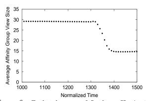
Figure 6: Fault-tolerance of Lookups II: At time t=1300, 500 out of 1000 nodes in a 30 affinity group system fail. This plot shows that failure detection and view (and hence filetuple) stabilization occurs by time t=1380.
