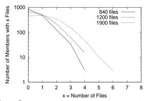
Figure 2: Load Balancing I: Number of nodes (y-axis) storing given number of files (x-axis), in a Kelips system with 1500 nodes (38 affinity groups).
