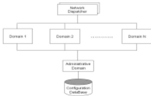
**Figure 1. Topology of the Océano prototype server farm.**
