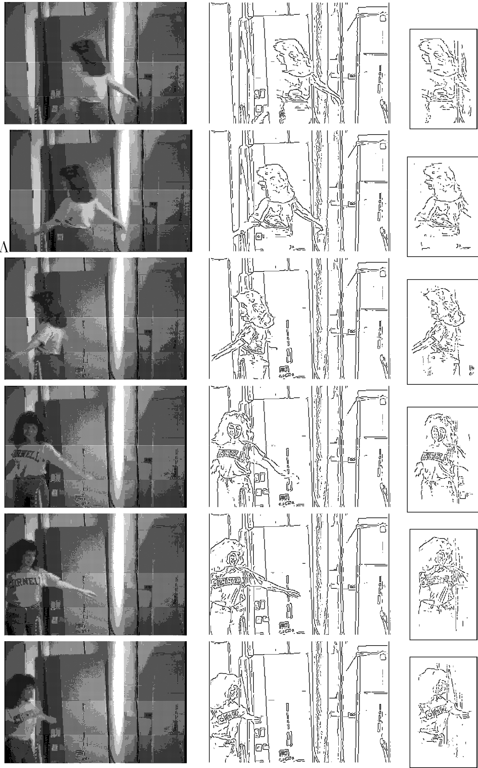
Figure 2: Six successive frames (numbers 14-19) from the same 100 frame motion sequence, and the corresponding models of the object being tracked.
