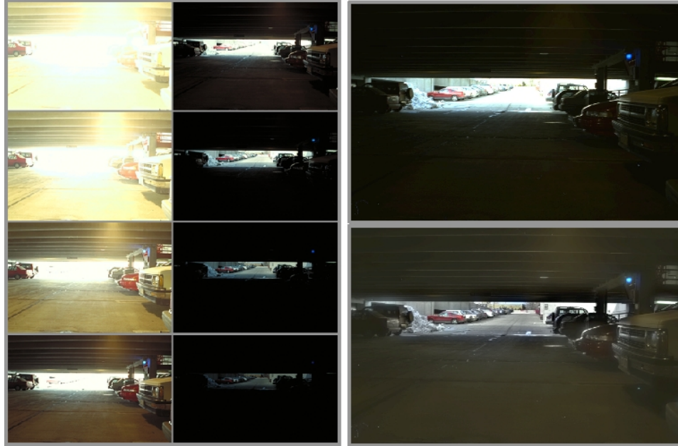
Figure 9: Tone reproduction of high dynamic range scene Left: Pictures taken at varying exposures Top Right: Direct linear mapping Bottom Right: Visual mapping
