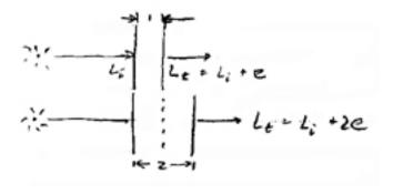
The generalization is that for a ray that travels through d units of a constant emissive medium, the resulting radiance  $L_t = L_i + de$ , a linear growth with distance:
