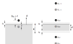
Figure 1: Dipole configuration for semi-infinite geometry (left), and the multipole configuration for thin slabs (right).
