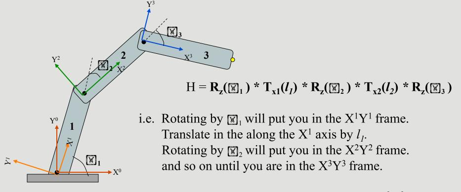
The position of the yellow dot relative to the  $X^3Y^3$  frame is  $(l_1, 0)$ . Multiplying H by that position vector will give you the coordinates of the yellow point relative the  $X^0Y^0$  frame.
