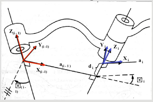
IDEA: Each joint is assigned a coordinate frame. Using the Denavit-Hartenberg notation, you need 4 parameters to describe how a frame (i) relates to a previous frame (i-1).
