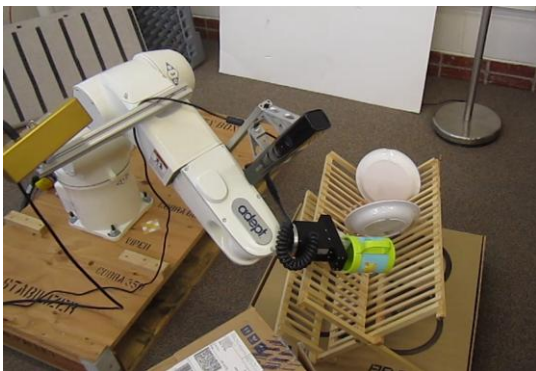
Figure 15: Adept Arm placing dishes into Wooden Slanted Dish Rack
