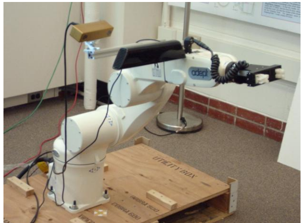
Adept Viper s850 arm with Gripper and mounted Microsoft Kinect
