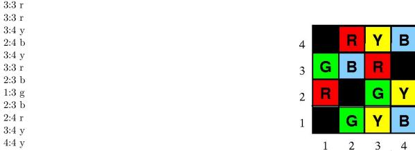
Here, the robot begins in square 3:3 perceiving red, attempts to make an illegal move (to the right), so stays in 3:3, still perceiving red. On the next step, the robot moves up to 3:4 perceiving yellow, then left to 2:4 perceiving blue (erroneously), and so on.
