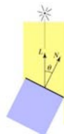
In general, light per unit area is proportional to \cos \theta = \mathbf{L} \cdot \mathbf{N}
