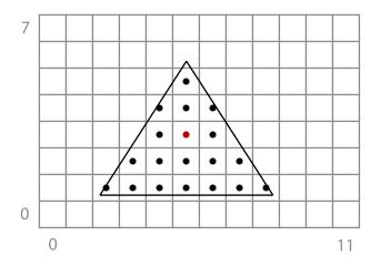
The camera's image is shown in the illustration above. Assume that the rasterizer interpolates screen-space barycentric coordinates to determine which fragments to generate, and that it is supporting z-buffering. In addition, suppose that the triangle is to be texturemapped, and that the vertices have texture coordinates  $(u, v) = (0, 0), (1, 0), \text{ and } (\frac{1}{2}, 1)$ .
