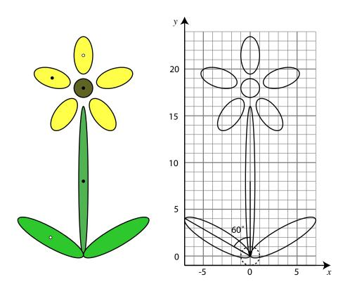
This drawing of a flower is made up of nine ellipses. These shapes can be thought of as instances of the unit circle, each transformed by a different 2D affine transformation. The major and minor diameters of the ellipses are all integers. All the parts centered on the y axis have integer or half-integer center points.
