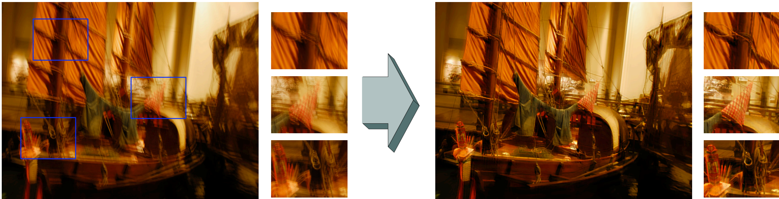
Figure 1 High quality single image motion-deblurring. The left sub-figure shows one captured image using a hand-held camera under dim light. It is severely blurred by an unknown kernel. The right sub-figure shows our deblurred image result computed by estimating both the blur kernel and the unblurred latent image. We show several close-ups of blurred/unblurred image regions for comparison.
