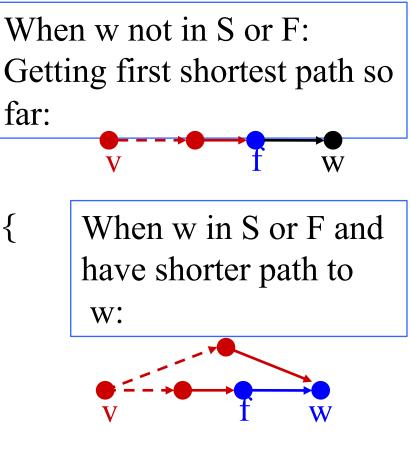
S **Far off** F S= { }; F= {v}; d[v]=0;while  $(F \neq \{\})$  { f= node in F with min d value; Remove f from F, add it to S; **for** each neighbor w of f { if (w not in S or F) { d[w] = d[f] + wgt(f, w);add w to F; bk[w] = f; else if (d[f]+wgt (f,w) < d[w])d[w] = d[f] + wgt(f, w);bk[w] = f;}
