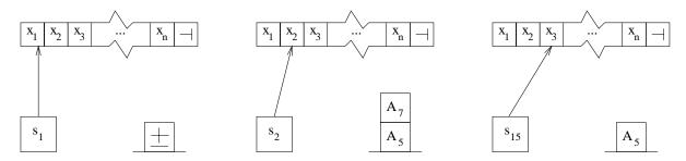
P accepts x if it can start in the initial configuration corresponding to x and, following its rules, have the input head fall off the input tape while changing to its accept state. If it would halt in any other configuration, such as getting stuck somewhere on the tape because no rule applies or falling off of the end of the tape but not in the accept state, it does not accept x.
