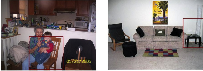
Figure 6: Example detections for the four component chair model. The left image is a true detection (despite heavy occlusion) and the right image is a false positive.
