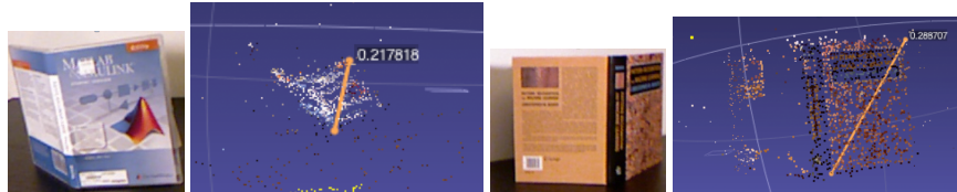
Figure 3: A 3D point cloud generated from depth-augmented bundle adjustment. Left: Correct size is 0.22 meters, Right: 0.30 meters.
