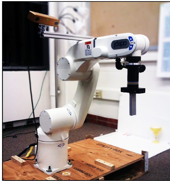
Figure 1: Adept Viper robotic arm with mounted Bumblebee stereo camera
