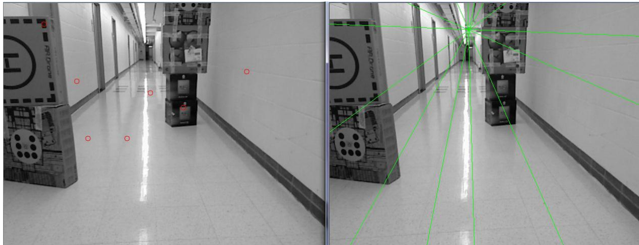
Figure 6: Point – Line Correspondence in subsequent images
