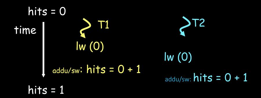
Timing-dependent failure  $\Rightarrow$  race condition
