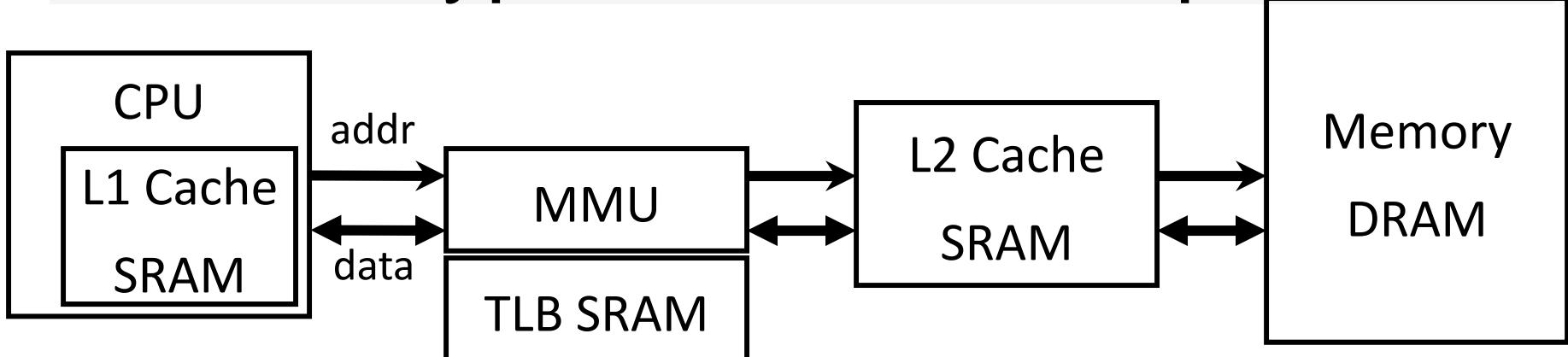
Typical L1: On-chip virtually addressed, physically tagged
