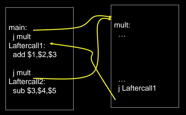
Jumps and branches can transfer control to the callee (called procedure) Jumps and branches can transfer control back
