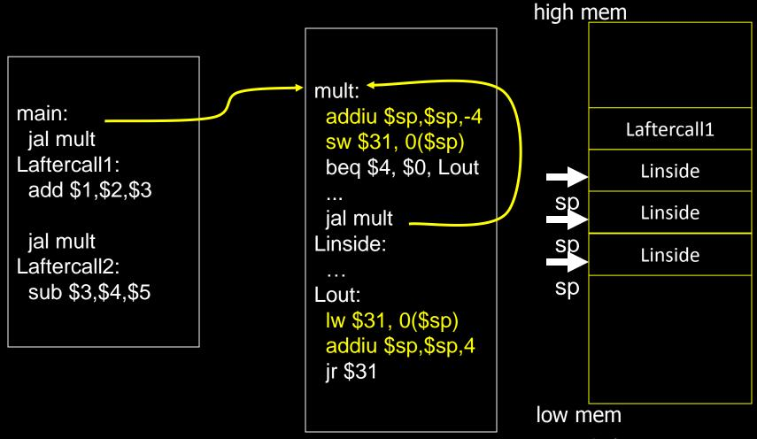
Stack used to save and restore contents of \$31
