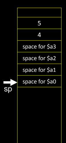
First four arguments are in registers The rest are on the stack There is room on the stack for the first four
